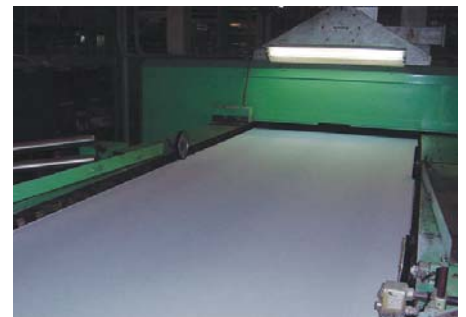
▲ top left: shirts/school uniform bottom: drying the textile after dipping into Photocatalyst solution
